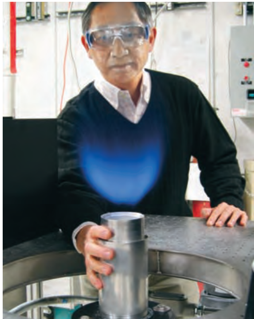
Figure 8. The low-swirl burner remains cool to the touch because the lifted flame does not heat up its body. The lifted flame originally was thought to be highly undesirable because in other burners it leads to unstable flame behaviors. But the unique divergent flow field of the LSB allows the lifted flame to self-adjust and remain robust even with a very lean fuel mixture.
