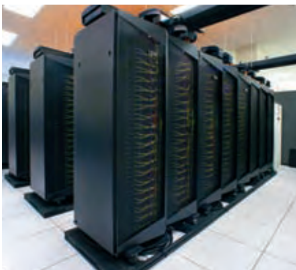
Figure 5. The Magellan system at NERSC will be IBM’s newest iDataPlex dx360 M2 server, with 5,760 Intel “Nehalem” cores and a theoretical peak speed of more than 60 teraflops. The system will be available to users in early 2010.
