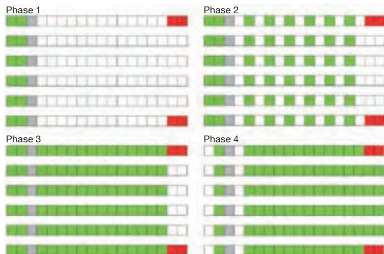
Figure 2. Four intermediate stages of the Franklin quad-core upgrade. The boxes represent Franklin system cabinets: white boxes for cabinets with dual-core nodes, green boxes for quad-core nodes, red boxes for cabinets containing both service nodes (which remained dual-core) and compute nodes, and gray boxes for columns in the NERSC machine room. Nodes were upgraded in place while Franklin remained in service for the users. Note that in Phase 4, NERSC exchanged the dual-core nodes located between the "red" service nodes with previously upgraded quad-core nodes to minimize downtime to users. In the final configuration (not shown), the last remaining dual-core nodes were upgraded with quad-core.
