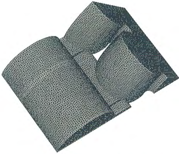
Figure 1a. The mesh for the Next Linear Collider Damped Detuned Structure cell.
