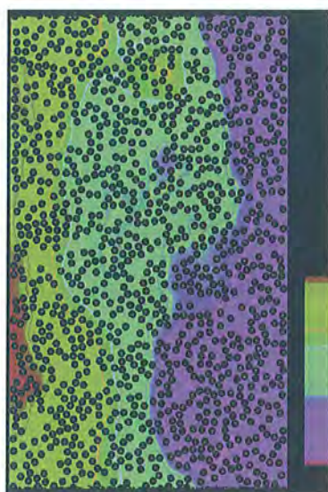
1,109 particles flowing in a Newtonian fluid in a channel. The mixture is pumped upwards against gravity. The color shows the stream function.
