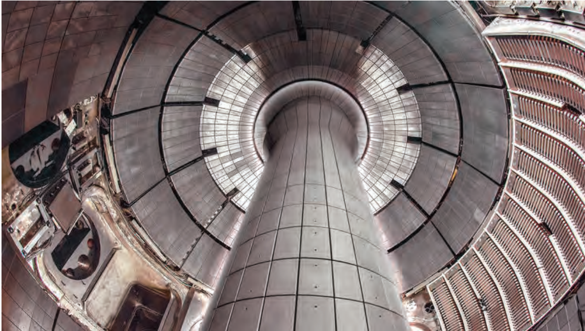
Figure 12. A series of simulations performed at NERSC show that the unique shape of the NSTX-U tokamak may help it disperse exhaust heat over a wider area on the material wall, making it a promising candidate for a pilot plant by the year 2040 in combination with other design features.
