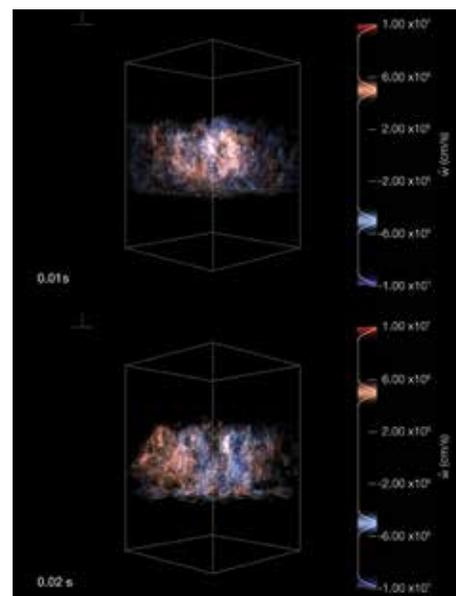
Volume renderings of the vertical velocity field at  $t=0.01$  s (top) and  $0.02$  s (bottom) for the wide calculation. Upward moving fluid is in red and downward moving is blue. *Image: Michael Zingale, Stony Brook University*
