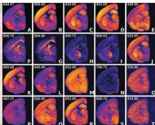
Ion-intensity visualization of the 20 most important ions in a mouse brain segment selected by the CX/CUR algorithm. Of the 20 ions, little redundancy is present, pointing to the effectiveness of the CX approach for information prioritization.
