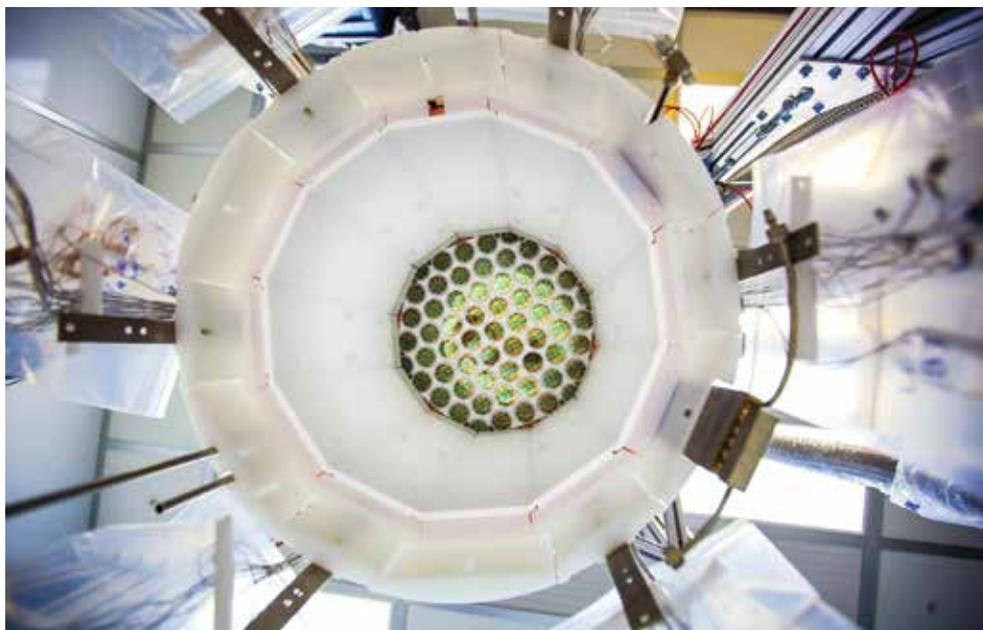
A view inside the LUX detector. Photomultiplier tubes can pick up the tiniest bursts of lights when a particle interacts with xenon atoms. *Image: Matthew Kapust, Sanford Underground Research Facility*
