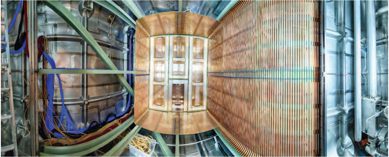
Figure 10. A prototype cryostat with 35-ton capacity is part of the infrastructure needed for the DUNE project.
