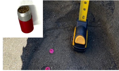
Sample Collection (diameter - 11 mm, length - 22 mm )
